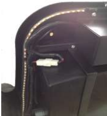
Alarm connector located under the floor deck front right.
